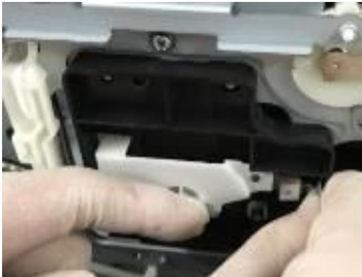
Check that the optical sensor for the maintenance home position flag is connected correctly (especially if the unit was recently removed or replaced)
