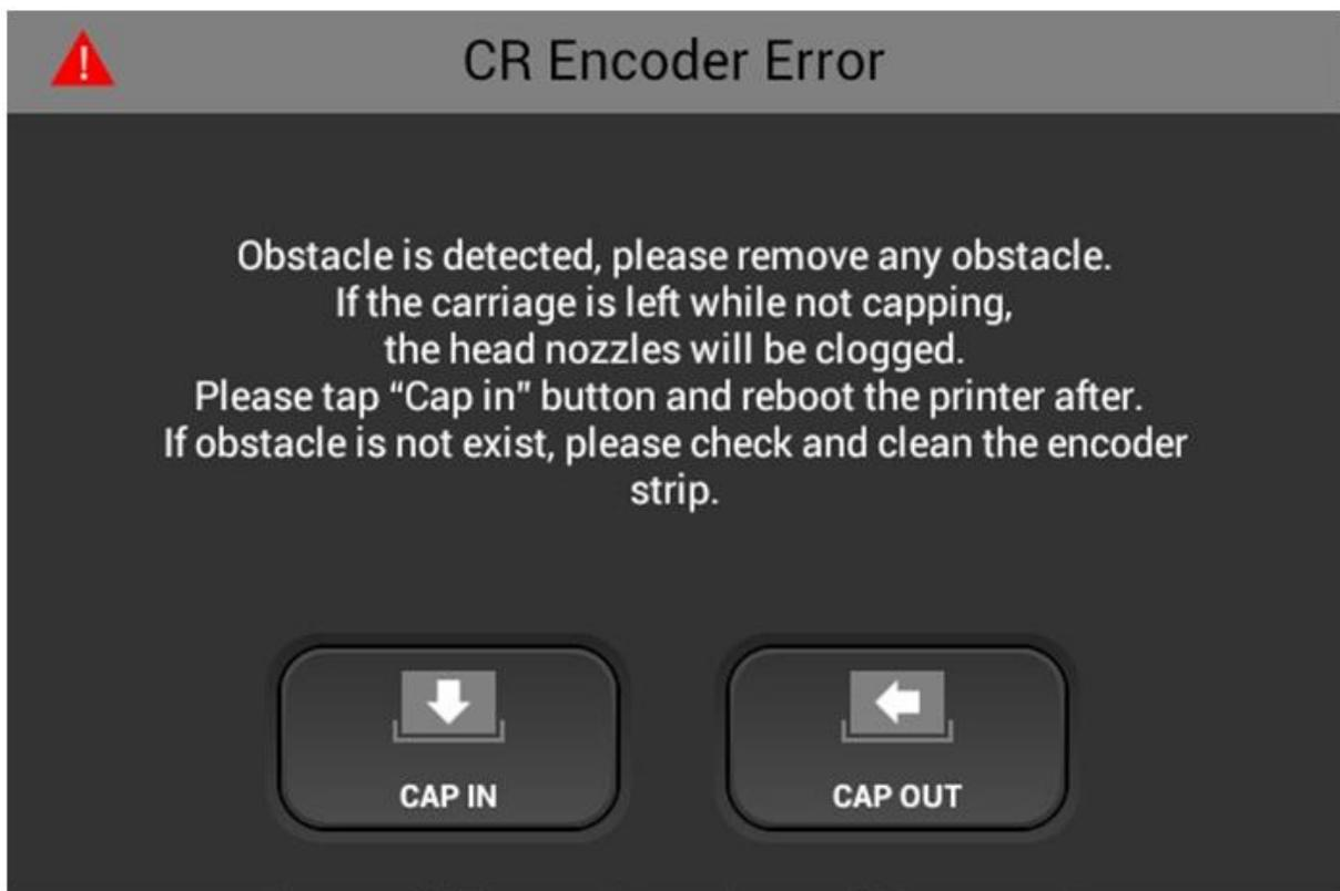
Check - for obstruction blocking carriage – Encoder not dirty or scratched – Encoder is installed in the carriage correctly. (especially if maintenance such as carriage or encoder replacement have happened)
