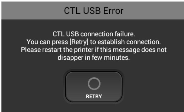
If this can not be reset by retry or power off and then back on – check the connection of the USB cable from the display assembly to the CTL board (see wire diagram) – also check the ribbon cable to CN 114 - this has the power signal to the CTL or check the memory prom on the back of the CTL to see if is installed correctly. If all connections are OK you may have to exchange the CTL board.
