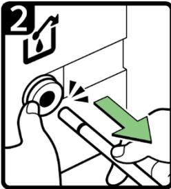
**IMPORTANT!** Do not pull the waste ink tube without pushing the plastic ring.
