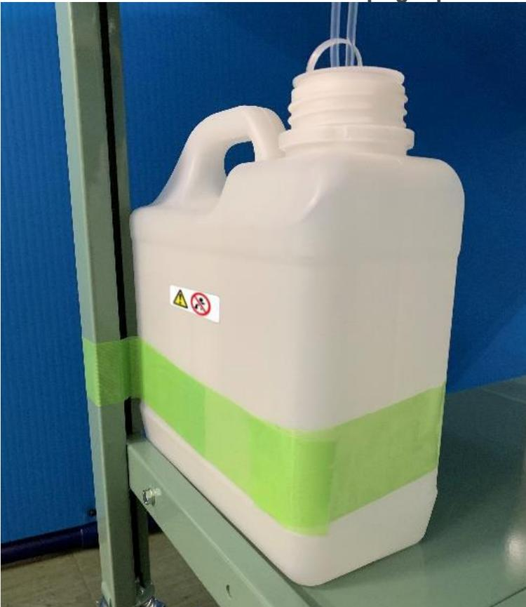
**IMPORTANT!** Install the waste ink bottle vertically. If installed horizontally, the waste ink inside could leak out.
