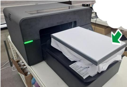
**IMPORTANT!** Make sure that the garment does not stick out of the lower frame of the platen.
