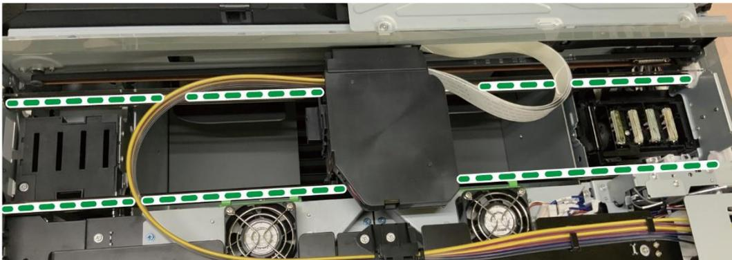
3. Move the carriage to the left, and then wipe off any old grease and lint on the guide rods where the carriage had stopped.
