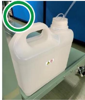
**IMPORTANT!** Connect the waste ink tube straight to the waste ink bottle. If the waste ink tube is bent or twisted, ink could become clogged inside the tube and thus could cause a malfunction.
