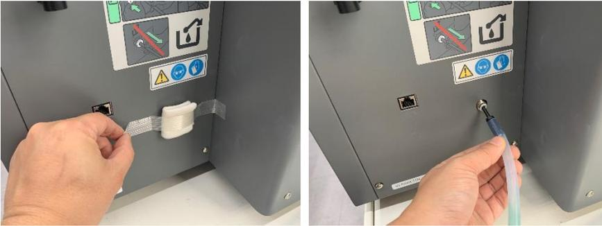
**IMPORTANT!** There is a marking on the waste ink tube. Insert the waste ink tube until the marking disappears into the waste ink bottle connector.
